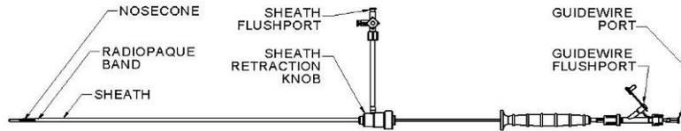
**Figure 4.** Schematic of TriVascular Ovation Abdominal Stent Graft System Iliac Limb/Iliac Extension Delivery Catheter
