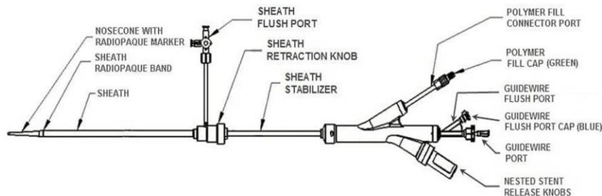
**Figure 3.** Schematic of TriVascular Ovation Abdominal Stent Graft System Aortic Body Delivery Catheter
